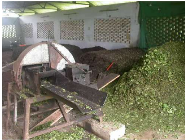
Fig.1. Composting unit showing a well ventilated hall and a weed chopping machine.
